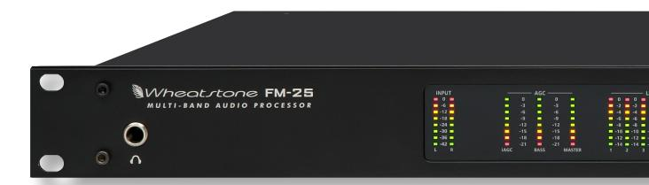
FM-25 is a multi-band audio processor ideal for LPFM or other FM stations requiring basic spectral audio shaping and peak limiting control.
